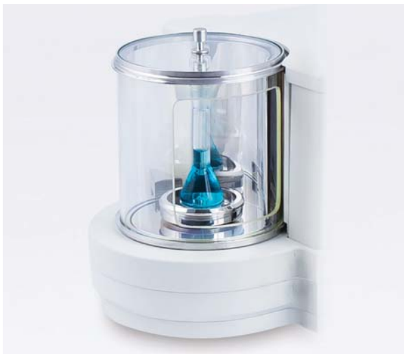
Using MYA 4Y microbalance for liquid weight measurement
